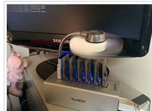
ASICMiner Block Erupter, a type of mining hardware used in 2013. [43]
